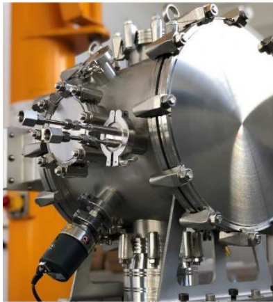
For small equipment Irradiation chamber to 150x150mm
